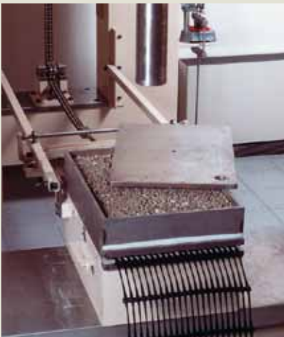
Shear test carried out in the laboratory of TENAX SpA.
